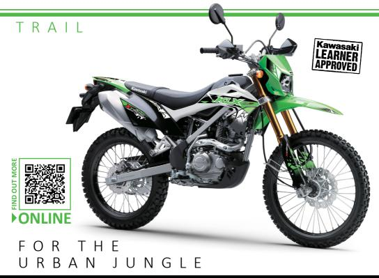
A simple yet reliable air-cooled single cylinder engine and highly rigid box-section perimeter frame are complemented by full-size diameter wheels. Inverted front forks offer an even higher level of off-road performance.
