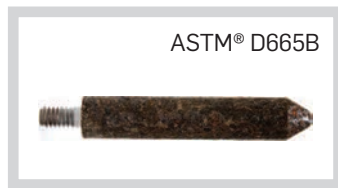
Treated with competitor's fuel stabilizer Extreme Rust
