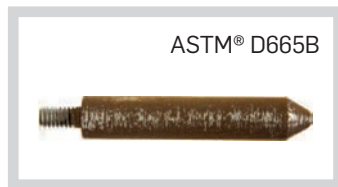
Treated with competitor's fuel stabilizer Rust
