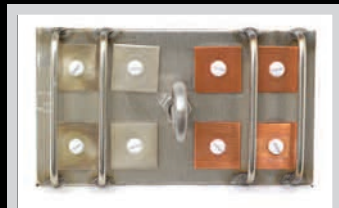
Treated with corrosion inhibitors found in Engine Med RX** Clean and Corrosion-Free
