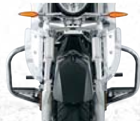
Cross Roads Lower Air Deflectors
