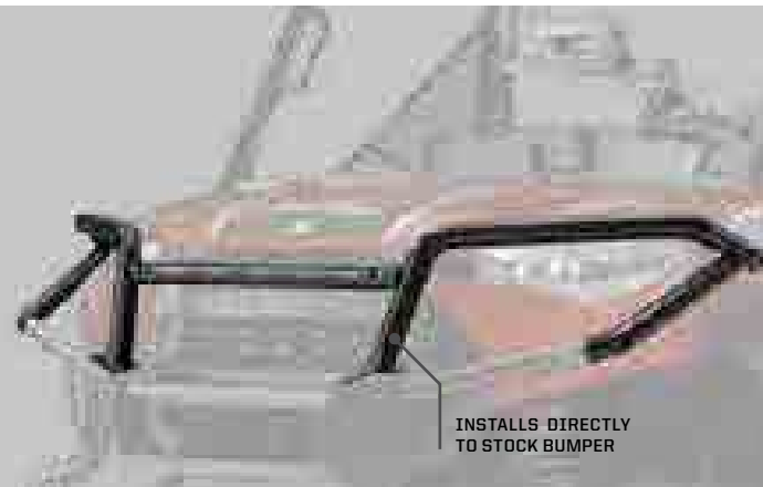
1 1/4" DIAMETER STEEL TUBE CONSTRUCTION
