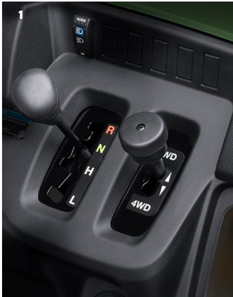
1. 2WD & 4WD Drive Modes 2. 12-inch Wheels and 26-inch Duro Tires 3. Ladder-type Steel Tube Frame
