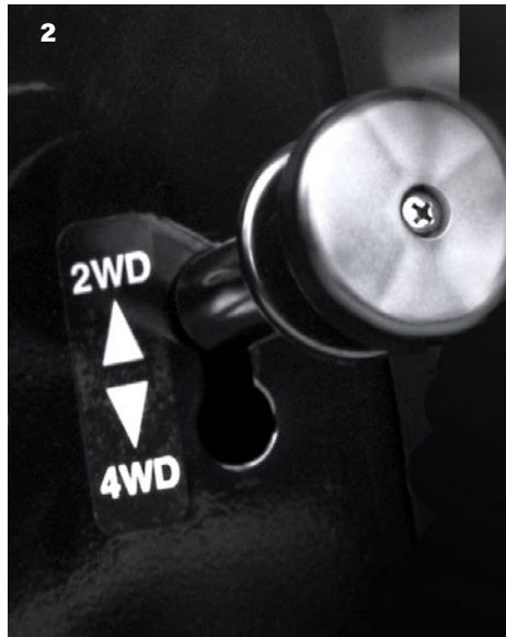
1. Fuel-injected V-twin Engine 2. 2WD/4WD and Dual-mode Rear Differential 3. MacPherson Strut-Type Front Suspension
