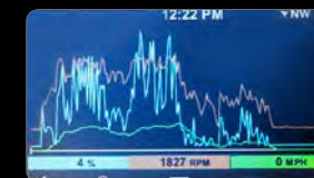
TPS, RPM and ground speed playback for up to 1:30 seconds to easily change clutching specifications
