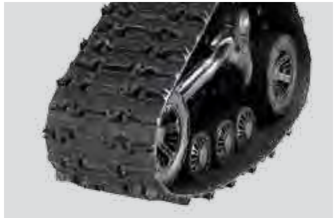
Heavy-duty, wide, rubberized wheels on a UHMW base to distribute the weight of the side-by-side
