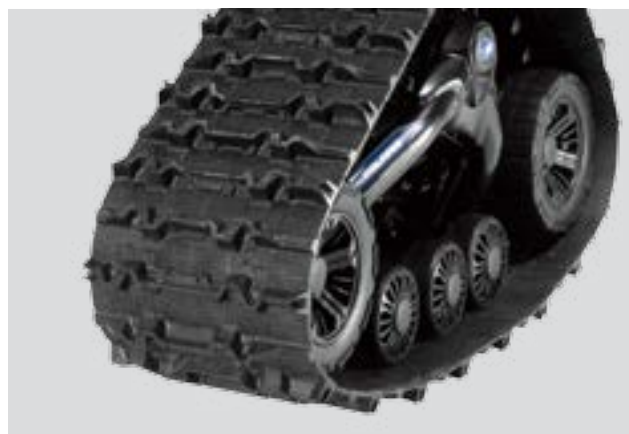
Heavy-duty, wide, rubberized wheels on a UHMW base to distribute the weight of the side-by-side
