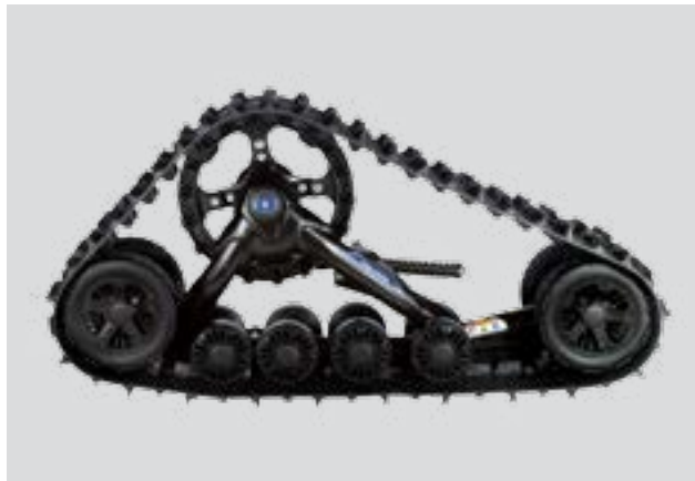
Exclusive Polaris' 20-18 tooth gear ratio, optimized for Polaris' drive train
