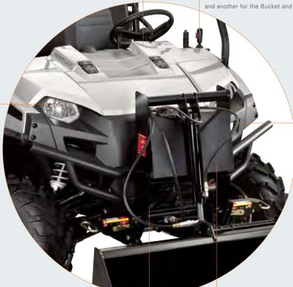
The large diameter connector pins in the Control Plug ensure a reliable electrical connection.
