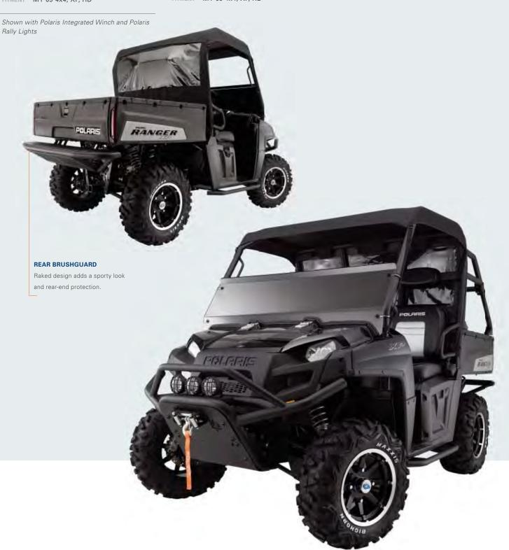
Plate steel construction features dual tow hooks, multiple winch configurations and auxiliary light mount options. Includes a heavy-duty bash plate. Late Fall availability.
